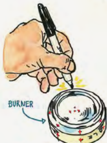
4. MAKE MARKS FOR HOLES ON BURNER PIECE
